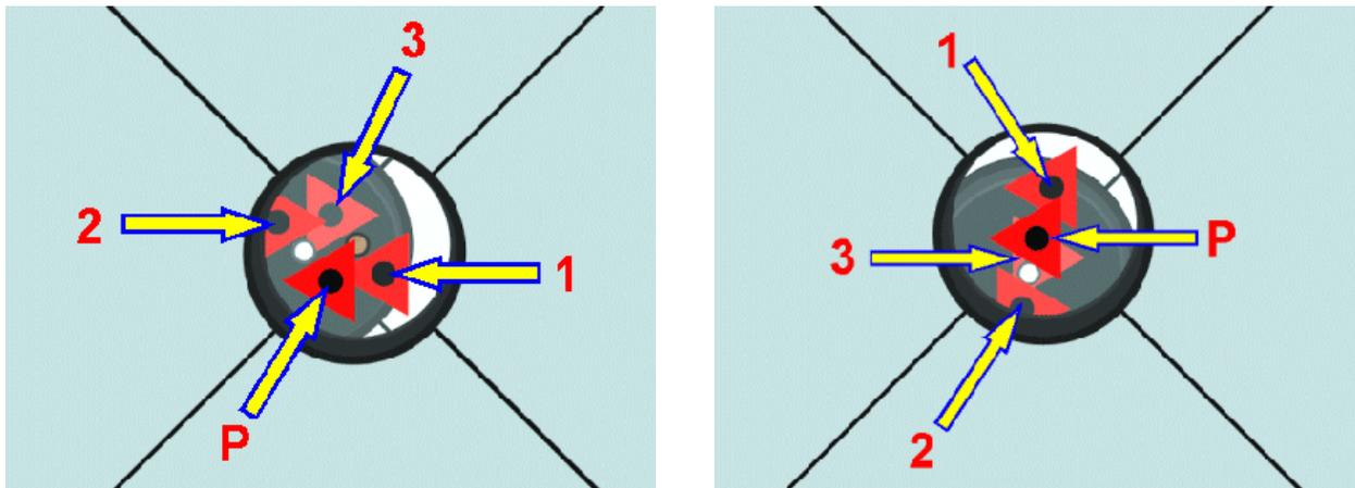
▲ **Reflection "P"** is the "Primary" or "first" reflection and is the direct reflected image of the spot itself via the Diagonal mirror after 1 FL pass. Reflection "P" is what is visible "without" the autocollimator whereas images (#1, #2, & #3) are reflections of "P"
